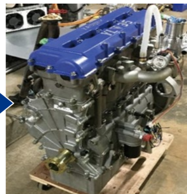
Built-in engine (3,500cc (four cylinders))
